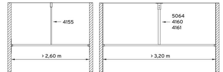
This picture shows when a 'strut-hanger' (5064) or V-hanger (4160/4161) is used and when a vertical suspension hanger (4155) is sufficient.
