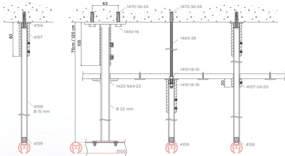
ceiling fixing with suspension hanger 4155
